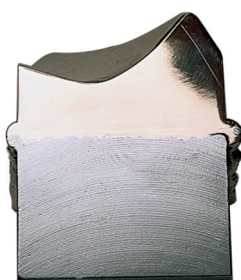
Section of electron beam welded wormwheel rim and centre showing the fusion of the bronze wormwheel rim onto the cast iron centre. This high security fit allows transmission of power under shock load conditions.
